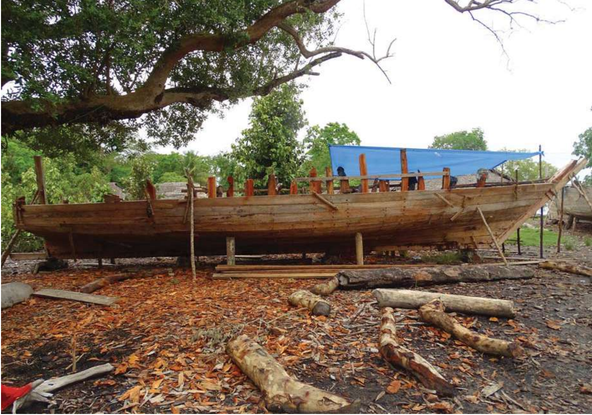
Boat making from mangrove wood in Rufiji Delta. ©Mwita M. Mangora
