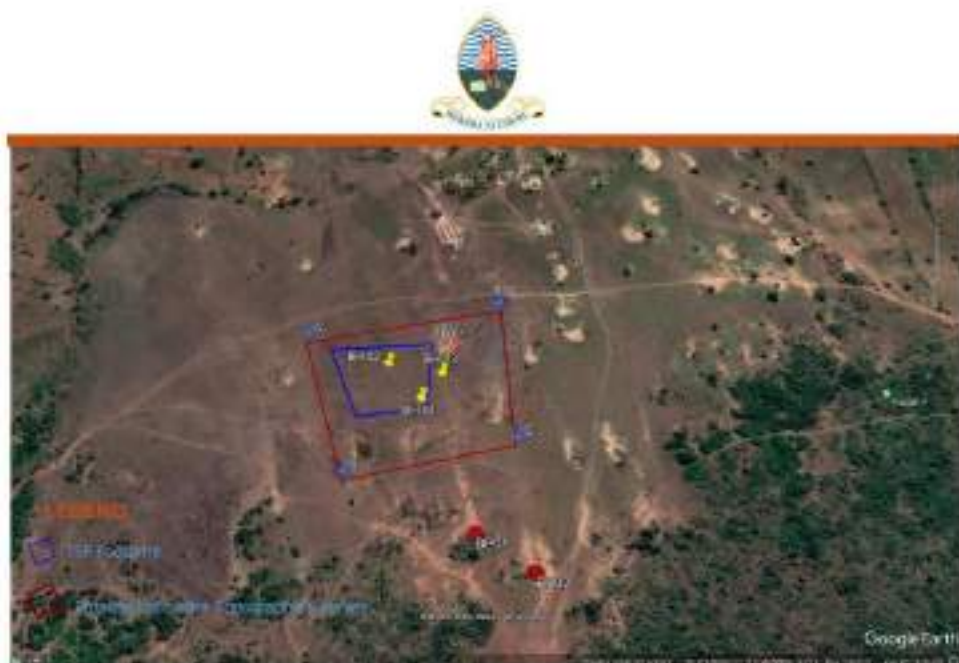
Figure 2: Google earth image showing the site of the proposed design of Tailings Storage Facility (TSF) at Bumva, Segese, Msalala, Tanzania with the relative locations of geotechnical investigation points and possible sources of soils for embankment clay lining.
