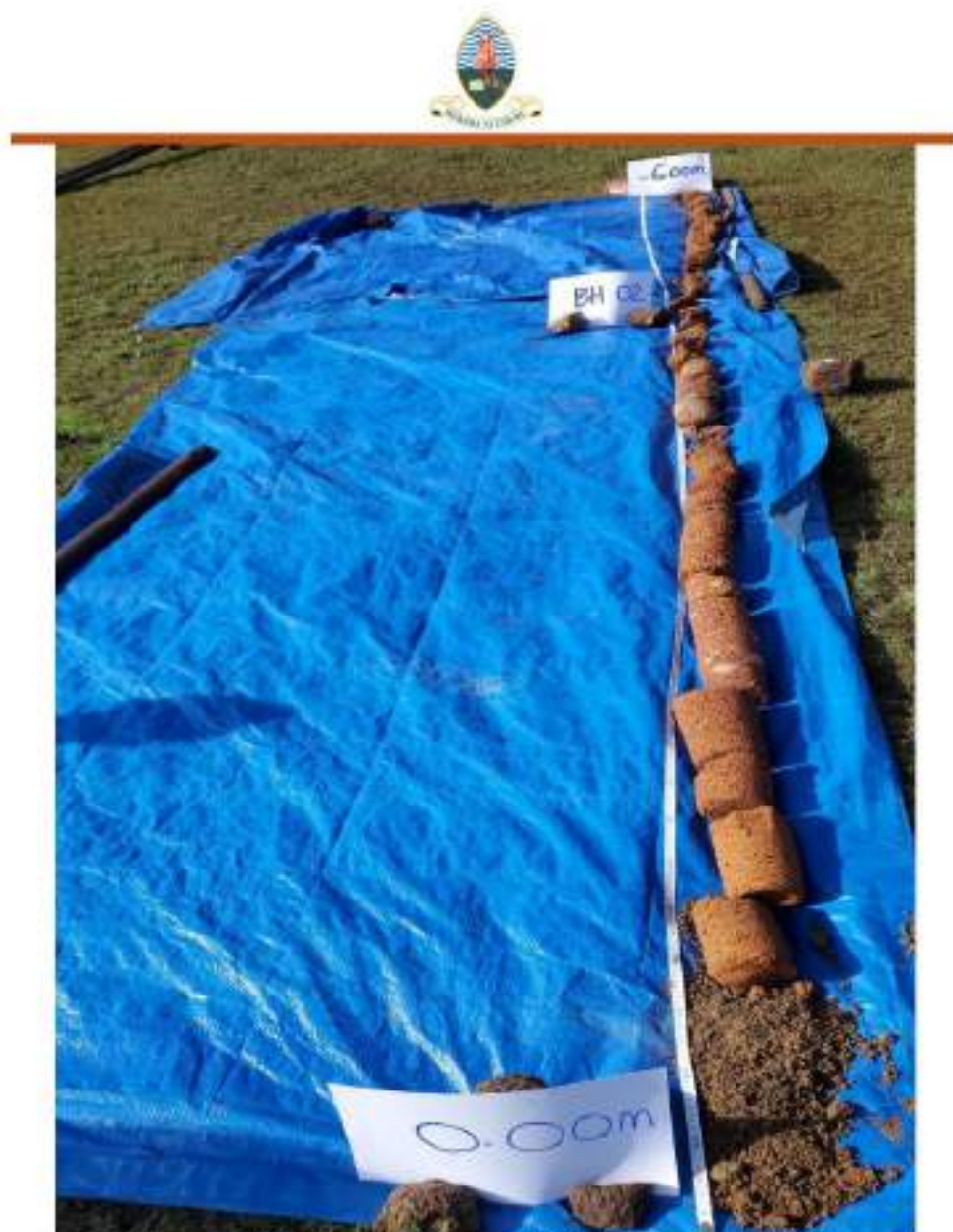
Figure 13: Image of ground profile from borehole BH02
