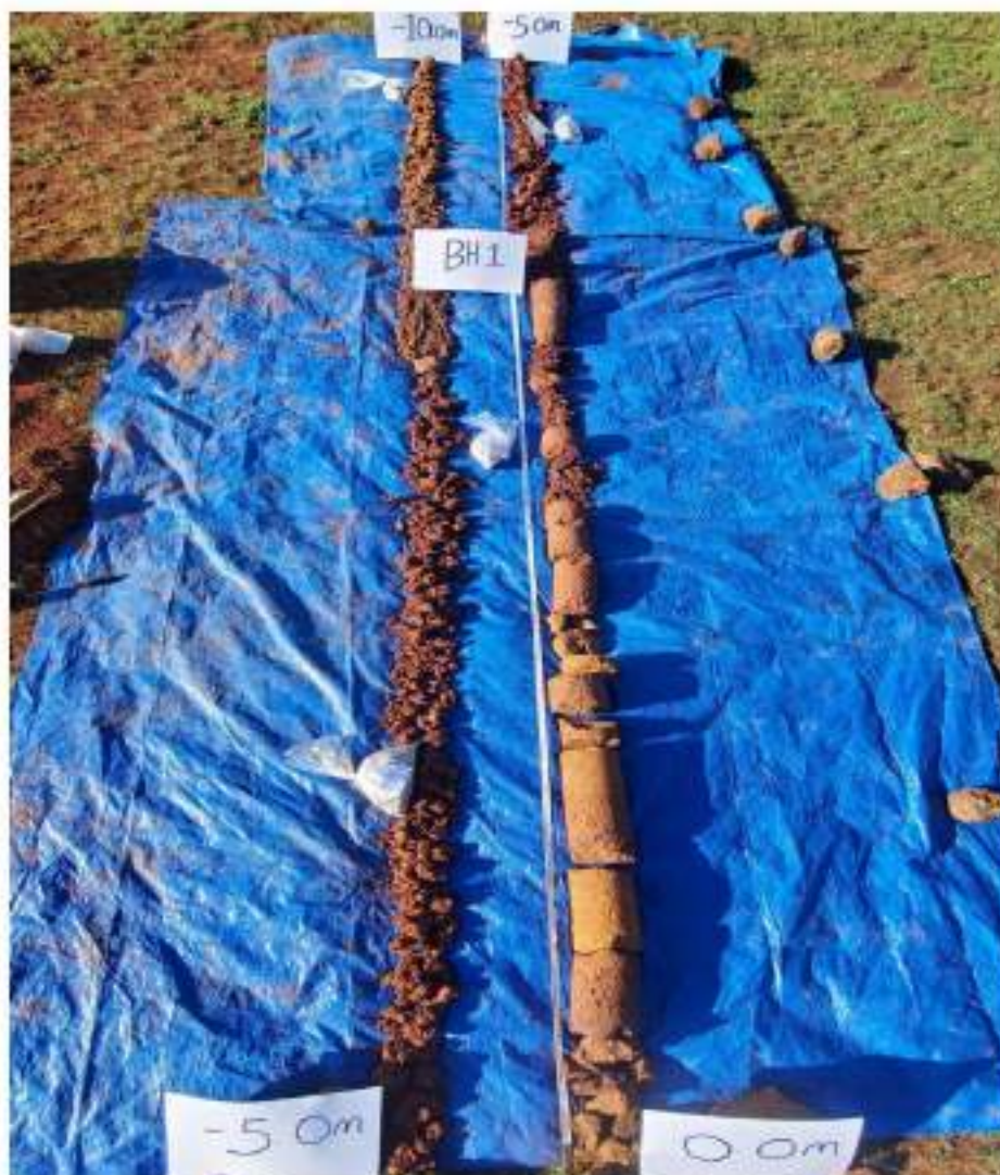
Figure 12: Image of ground profile from borehole BH01
