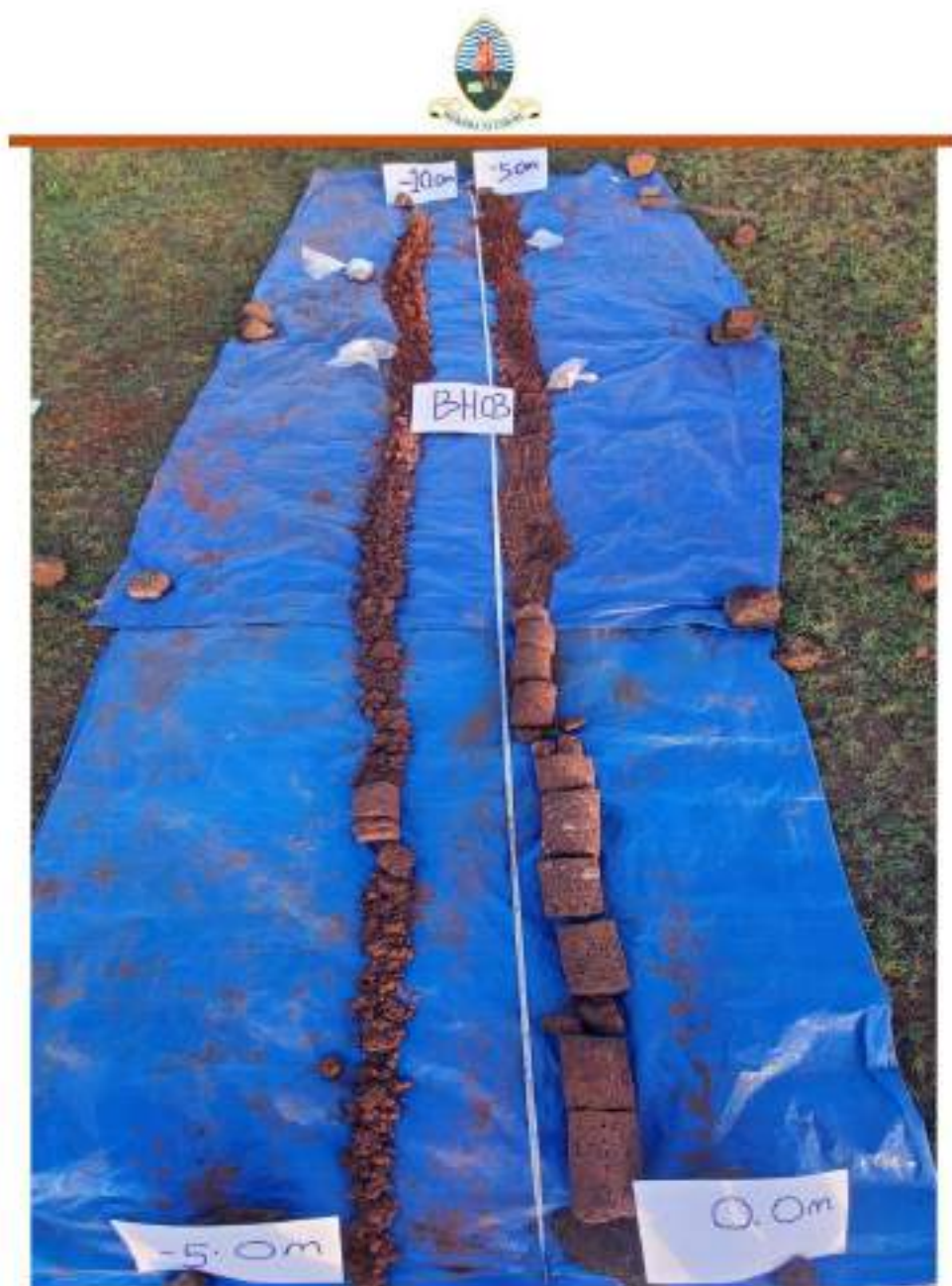
Figure 14: Image of ground profile from borehole BH03
